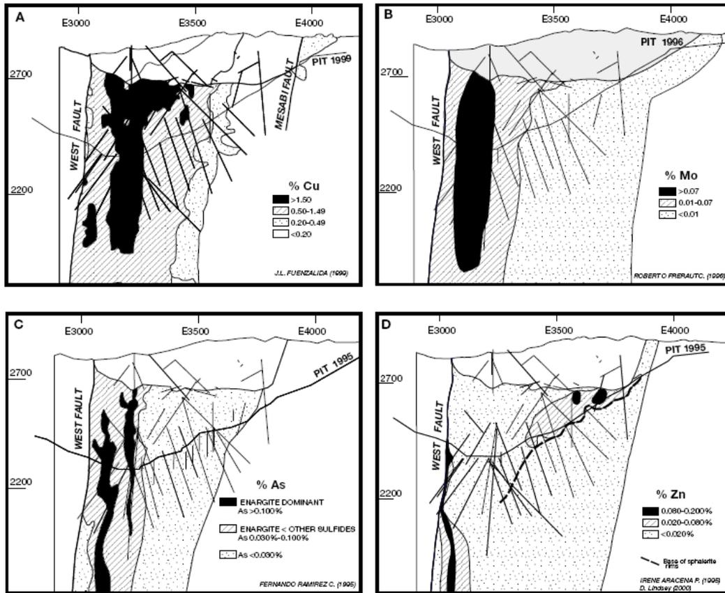
Fig 3: A-D. Distribution of copper, molybdenum, arsenic, and zinc in 3600N section, from diamond drill hole and blast holes. Reference: Ossandon et al. 2001, Geology of the Chuquicamata Mine: A progress report: Economic Geology, v. 96, p. 249–270.
