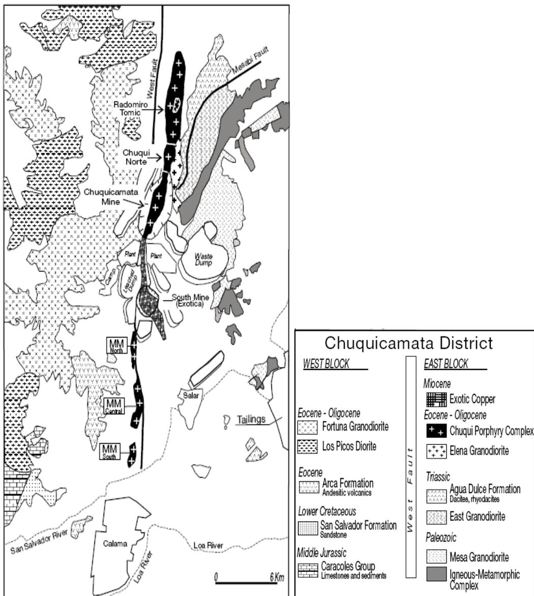
Fig. 1: The Chuquicamata district, showing major geologic units and location of mines. Geology is modified from G. Chong and R. Pardo, unpublished map (1997). The Chuquicamata mine is at 22°17.5' S, 68°54.5' W (UTM E510350, N7535600). Reference: Ossandon et al. 2001, Geology of the Chuquicamata Mine: A progress report: Economic Geology, v. 96, p. 249-270.
