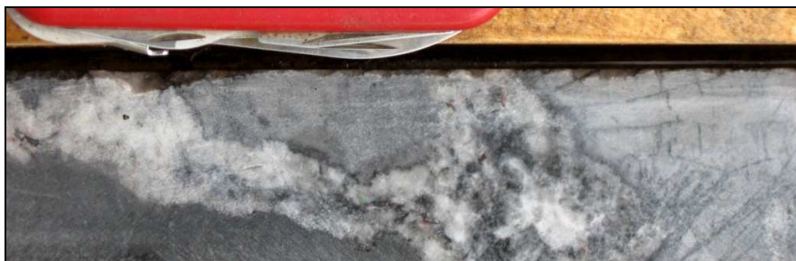
Fig.10. sparry calcite vein with speckles of chalcocite (drill core KCN7)
