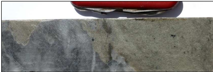
Fig.6. contact of the sandstone and light to medium grey dolostone (drill core AU12-245)
