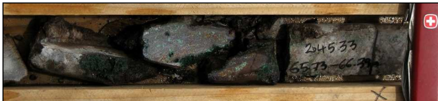
Fig.9. massive ore comprising bornite, chalcopyrite and malachite (drill core KCN7)
