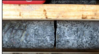
Fig.5. oolitic medium grey dolostone (drill core AU12-193)
